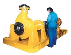
**Torque Ring Drive:** Also know as an Eddy Current Drive. A magnetic coupling consisting of a permanent outer magnet ring and an inner torque ring containing a network of copper rods supported on a mild steel core. The rotating outer magnet ring generates eddy currents in the copper rods, which converts the core to an electromagnet. The electromagnet follows the rotating outer magnet ring, but at a slightly slower speed due to slip, i.e. asynchronous drive.
