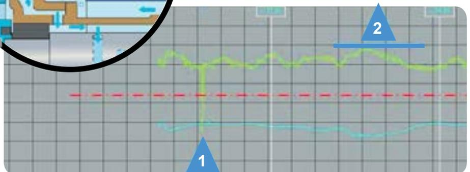
▲ Digital Control System data recorded by a VapourView user (Sealless pump on Pre-treater Stripper Reflux – Hydrocarbons) Potential gas event noted at **POINT 1**. This event passed, then generally a high mA signal in relation to the product temperature occurs at **RANGE 2**.
