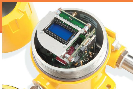
The VapourView® instrument provides vital information to the end-user on the presence of gases in the pump's internal flow regime and forewarns of adverse conditions likely to affect bearing lubrication or magnetic coupling cooling. Early intervention by system engineers, who can undertake remedial action, will maximize the operating life of plant equipment.
