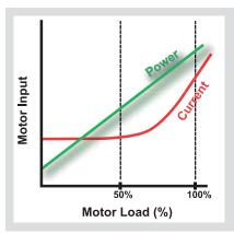
Power Monitoring has distinct advantages over common current monitoring, also known as amperage monitoring. The current is almost constant up to 50% of the motor load range and because of this, it is very difficult to detect changes below 50%. In contrast, because the input power varies linearly across the entire motor load range, it is an extremely reliable and accurate detector of system changes. As such, most pumping condition changes will be seen in input power fluctuations.
