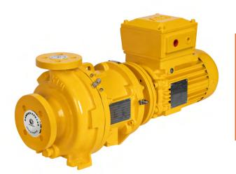
By completely eliminating the seal and associated seal support system, our pumps are ideal for handling any toxic or hazardous liquid. Applications include process, utility services, elevated suction pressures, sampling, fiscal metering/custody transfer, elevated temperatures, caustic, solvents, cooling, booster and heat transfer pumps.
