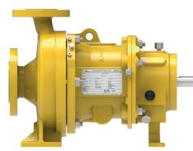
The CSI (ISO) frame 1 product line covers a hydraulic range that offers pumping solutions up to 22kW. The pumps are offered with a range of bespoke Synchronous Magnetic Drives rated to match prime mover performance and with both metallic or high efficiency ZeroLoss® containment shells as standard.
